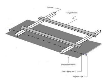
Guide for overlapping joints into wooden trusses:
